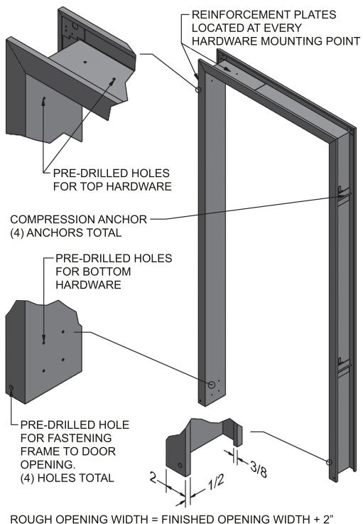
ROUGH OPENING WIDTH - FINISHED OPENING WIDTH + 2 ROUGH OPENING HEIGHT = FINISHED OPENING HEIGHT + .75"
